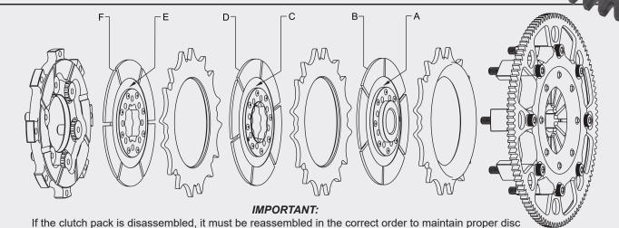
clearance. Each side of the discs is labeled with a letter—refer to the diagram to ensure accurate reassembly.
