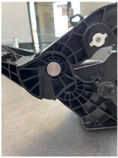
5. Place the clutch pedal arm back into the pedal assembly and slide the lubricated pin through the assembly and the clutch pedal arm. Make sure smaller diameter end goes in first. Clean up any excess lube that may have squeezed out during assembly.
