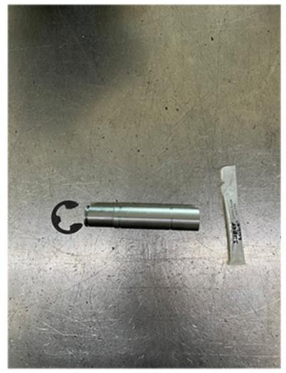
4. Prep the new clutch pedal pivot pin. Apply a small amount of the provided Super Lube to the length of the pin with the bigger diameter and the two grooves. There is no need to lubricate the smaller diameter section of the pin.
