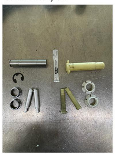
Comparison of new Clutch Master Billet pins and bushings vs. the OE plastic pins and bushings.
