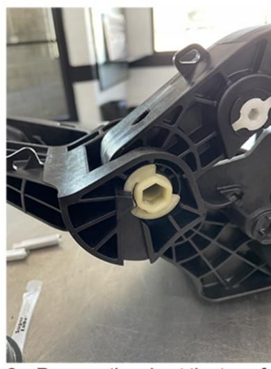
2c. Remove the pin at the top of the pedal that the clutch pedal pivots on. This pin uses a 10mm allen. Twist it 90deg to unlock the tabs and then it will slide out.
