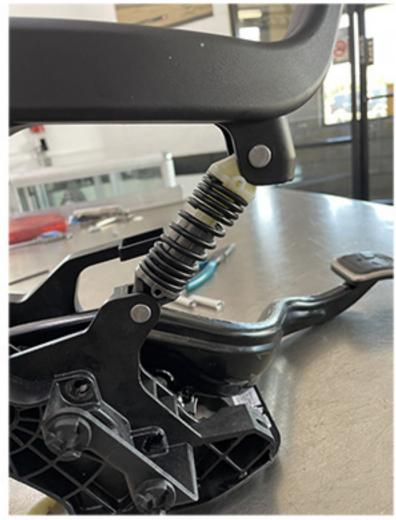
2b. Remove the return spring pins from either the pedal or the pedal assembly. Be careful not to loose the spring. It is not under a great amount of tension so it will not fly off.
