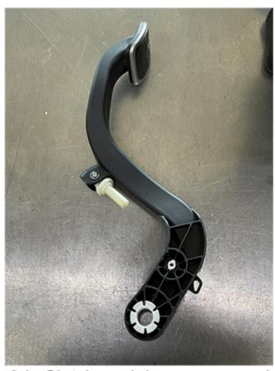
2d. Clutch pedal arm removed from clutch pedal assembly. Remove the two white plastic bushings from each side of the pedal arm.
