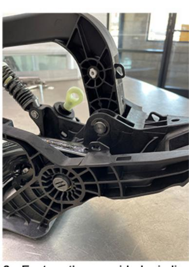
Fasten the provided circlip onto the groove on the clutch pedal pivot pin to lock the pin in place.
