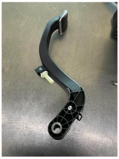
Press the new CM stainless steel bushings into the pedal arm.
