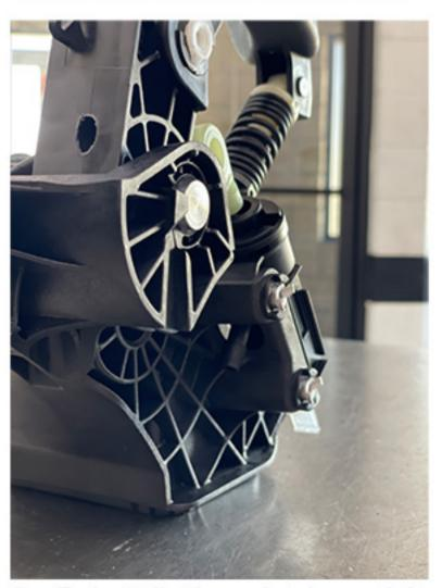
Reinstall the clutch pedal return spring and connect the master cylinder clevis back to the pedal arm.
