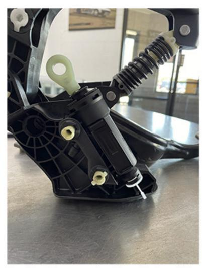
2a. Start by removing the clutch pedal. You will remove the two pins holding the master cylinder to the pedal assembly. These pins use an allen but can fairly easily be stripped so a TP40 also works. Twist the pins 90deg to unlock them and they will slide out.
