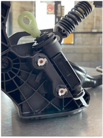
7. Reinstall the clutch master cylinder into the pedal assembly. It doesn't hurt to put a little bit of the Super Lube on the new aluminum pins to slide them into place. Once the pins are slide into place, use the 4mm allen to turn the pin 90deg tp lock them in place.
